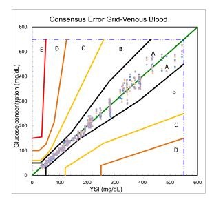
Results of error grid analysis demonstrated that 100% of the results fall in zone A which indicates the meters are clinical accurate.
